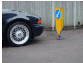
Figure 4 - Frangible obstacle: Minor traffic signal.
