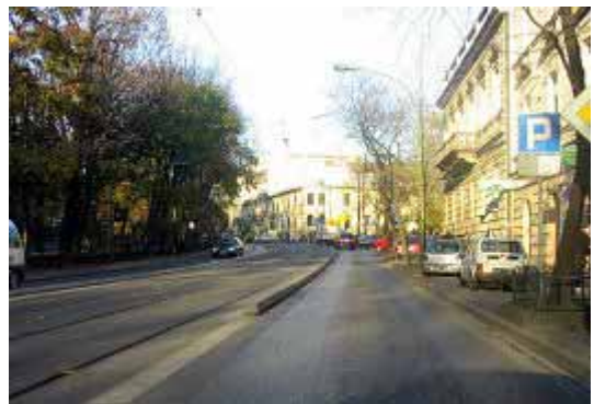
Figure 5 Kerb as a lane separator (width of the lane is 3,50m), (source: id.)
