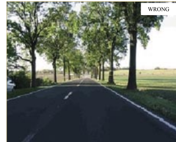
Figure 38: Invisible crossing in a tree-lined country road (300 m ahead). [22]
