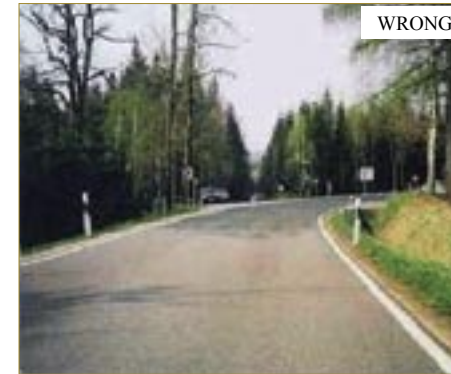
Figure 40: Optical irritation: roads course goes to the right contrary to the straight-ahead orientation line (150 m ahead). [22]
