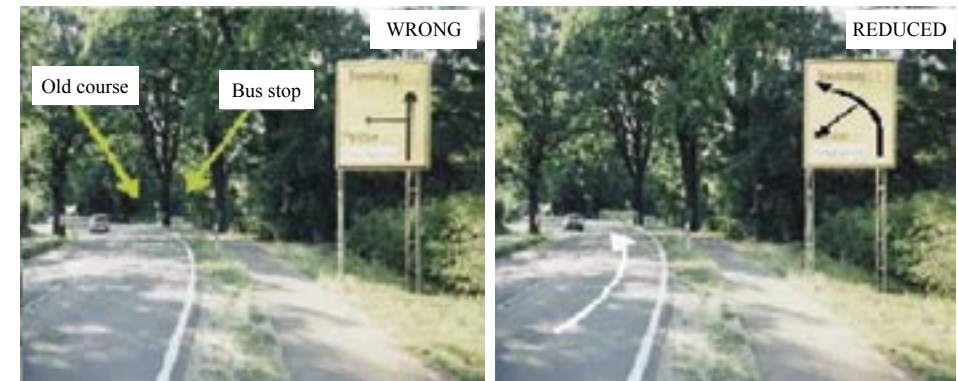
Figure 50: Traffic sign shows another direction than the present course. Some drivers try to follow the old course. [22]
