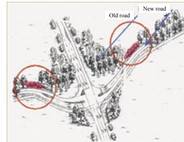
Figure 42: Change of road's course contrary to the dominant eye-line focus, corrected by planted embankment. [18]
