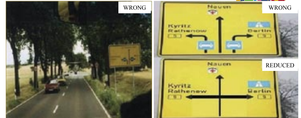
Figure 53: Corrected signing on the accident point. [16]
