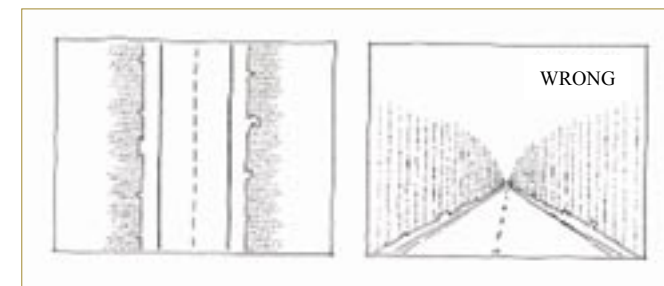
Figure 14: Optical density of the field of view is low; monotonous and long, straight-ahead approaching section leads the driver to speed up [15]
