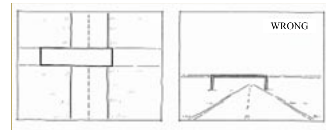
Figure 17: Lateral space structure: asymmetrical superstructure leads to confusion, driver drifts to the left lane [15]
