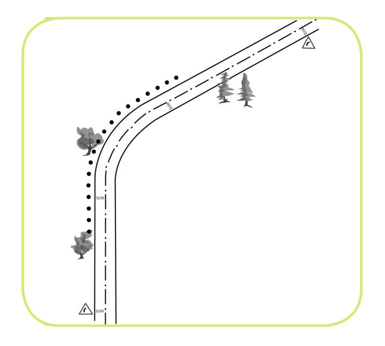
By joining the two finishing points together with a system of vergemasters, the plan will look like this.
