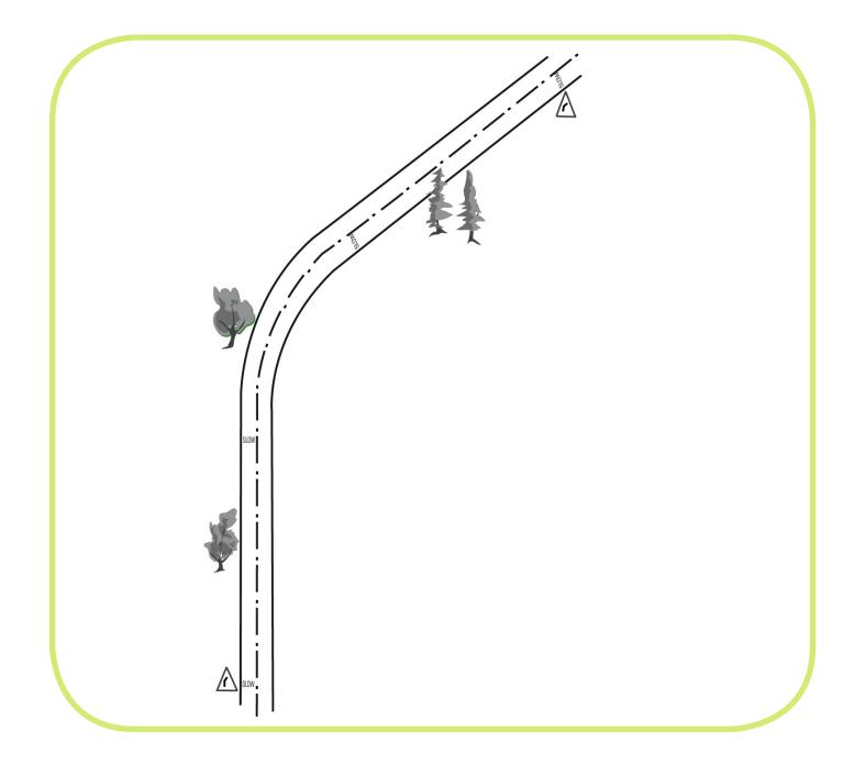
This is the plan view of the bend. It already has a bend sign reinforced by two slow sign in each direction. There are some trees that could be a cause of distraction.
