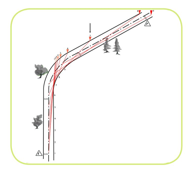
By drawing a straight line from the centre of the roadway to touch the inside edge of the bend and continuing that line till it touches the outside edge of the bend, as line No I, you can see in plan view where the theoretical vanishing point is for the position at cats eye No I should be.
