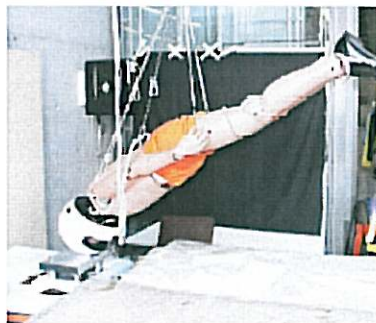
Drop test configuration for 30° and 90° impacts with an adult male dummy.
