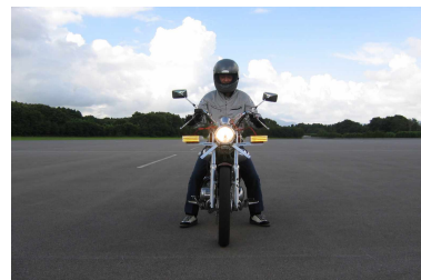
(8) Amber position lamps (80cd, 150mm) on + AHO
