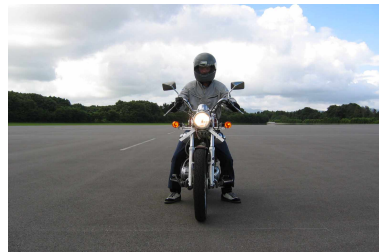
(6) Amber position lamps (30cd, 150mm) on + AHO
