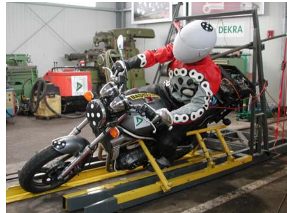
Figure 7. Test sled inclined impact with dummy and motorcycle.
