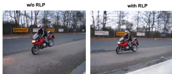
Figure 9. Motorcycle Integral Brake System (MIB) Rear wheel Lift-off Protection.
