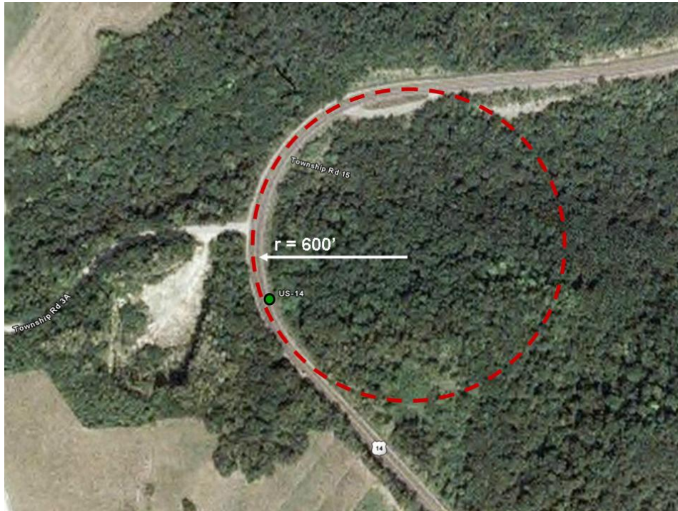
Figure 5. Orthoimage of Crash Site (on US-14) with Illustration of Approach for Measuring Radius of Curvature.
