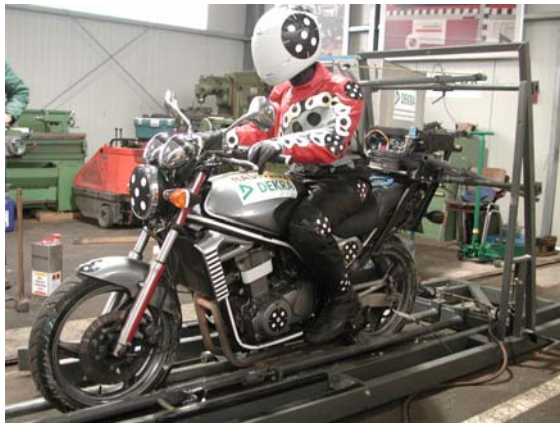
Figure 9. Test sled upright impact with dummy and motorcycle.
