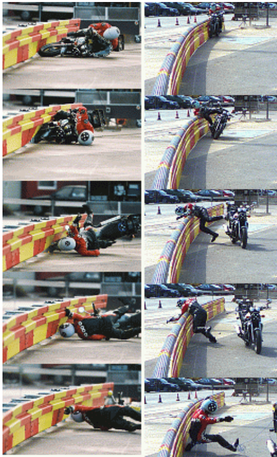
Figure 10. Motion sequence of inclined and upright crash test.
