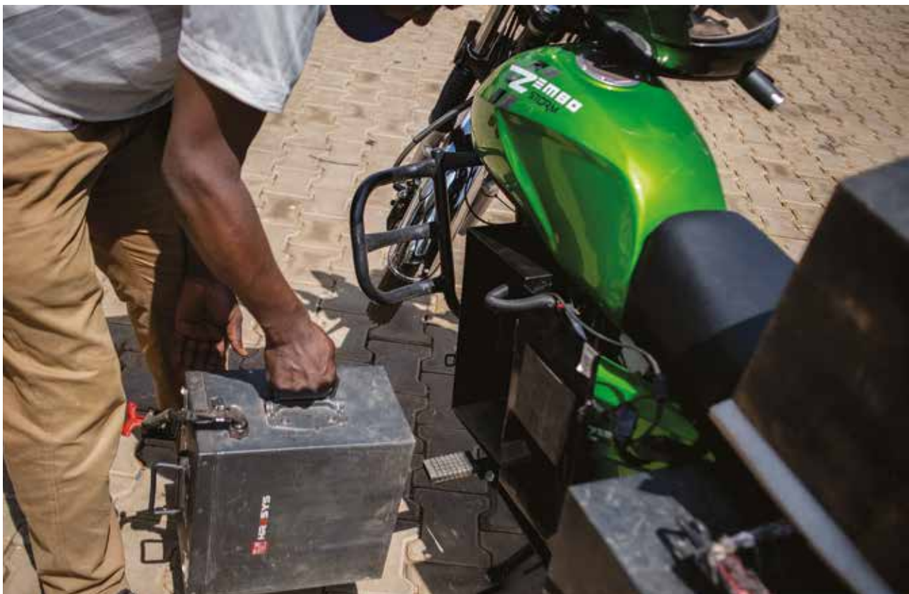
Changing a battery on a Zembo e-moto in Uganda
